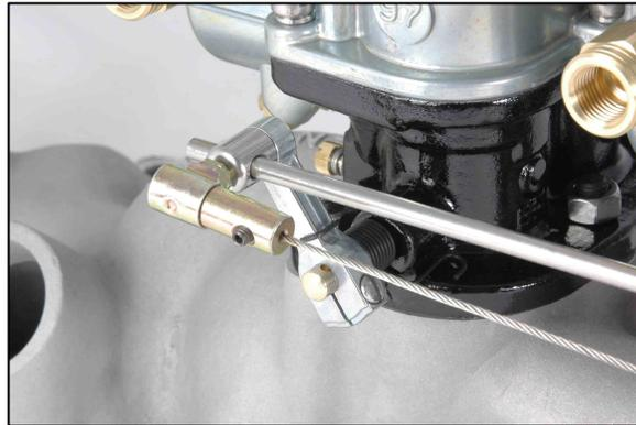
Install your cable kit onto the 9136K bracket as per the cable manufacturer's instructions. This usually just involves clamping the cable outer shield through the hole in the arm of the bracket. The arm is set at an angle to give the cable the optimum 'bind-free' pull on the linkage.
