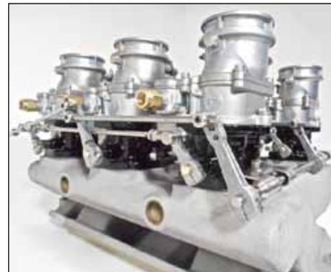
**TwoStep 6x2 Back-bar kit adjusted for parallel link rods at rest**
