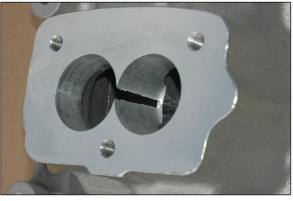
Your first task is to open out the carb intake ports to avoid a step under the carburetor. The BIG97 throttle barrels flare out to 1.4inch at the bottom of the base casting so that's what you're aiming for in the manifold.
