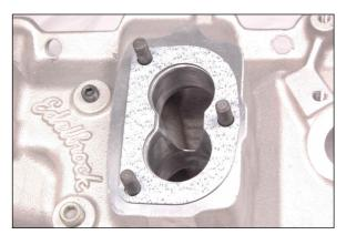
Extend the early plenum effect by cutting away that central web between the two barrels and smoothing the transition down into the plenum. The machining operation had already created a slot so we just used the die grinder to smooth around the edges and turn the slot into a V shape.
