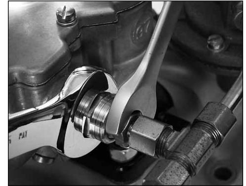
**CAUTION:** When connecting the fuel line, hold the S-jet inlet fitting (see above) with an 11/16-inch open-end wrench. This fitting must not be allowed to turn in the carburetor. If the fitting is allowed to turn, it could upset the pre-set float level adjustment, which can cause carburetor malfunction and flooding.
